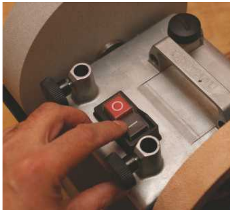
▲ Rubber-shrouded power switches are easily accessed. Note the solid zinc top and carry handle
